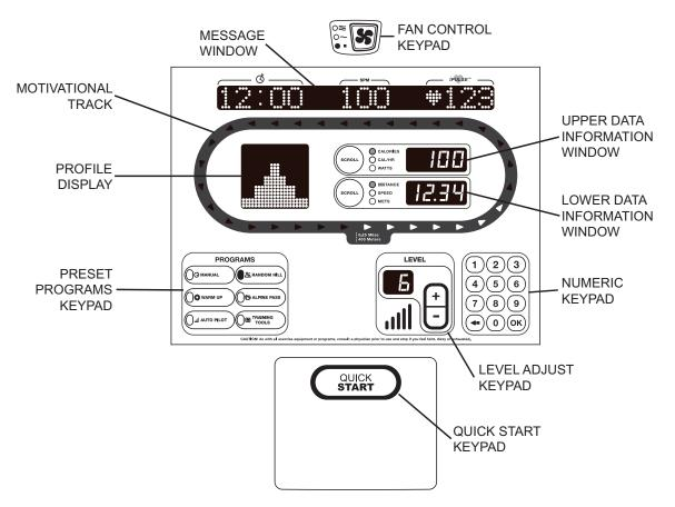
Upper Data Information Window: Shows current and aggregate data related to your workout. Pressing the associated SCROLL key scrolls between the following displays:
