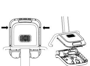
c) Slide the display console neck onto the neck brackets of the bike frame. **CAUTION:** Be careful not to pinch the wires or your fingers between the console neck and the bike frame when sliding the console into place.
