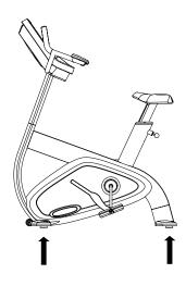
Place the bike on the floor in the position in which it will be used. Use the leveling adjusters (located on the underside of the front and rear feet) to compensate for uneven floor surfaces and to eliminate wobbling.
